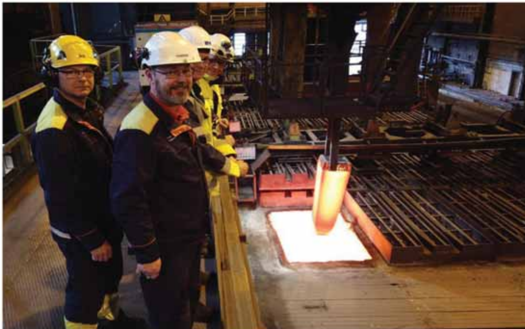
6 x 4.2 ton ingots per pit furnace, all same ball bearing steel grade
