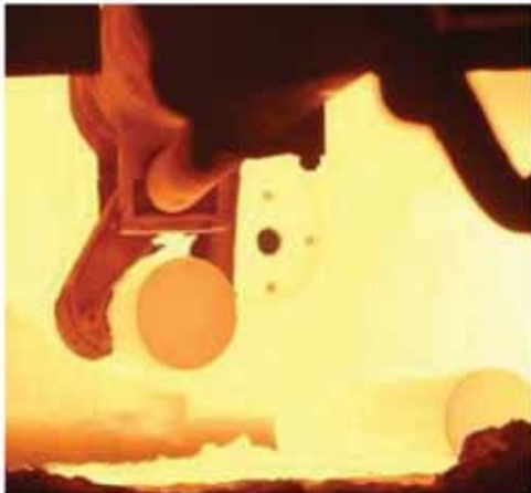
Natural Gas fired Flameless Oxyfuel at Rotary Hearth Furnace for Tube Production
