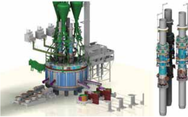
Fig. 6: TENOVA PYROMET Open Slag Bath Furnace. On the right: Soederberg type electrodes (TENOVA, 2019)
